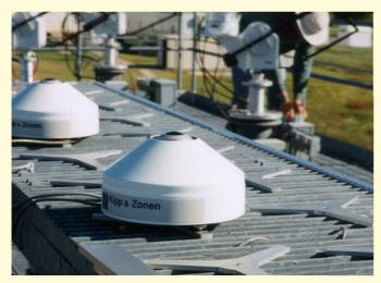
CV2 can be used under all weather conditions and is easy to use. The only part that needs maintenance is the removable air filter at the bottom, which should be checked at regular intervals.
